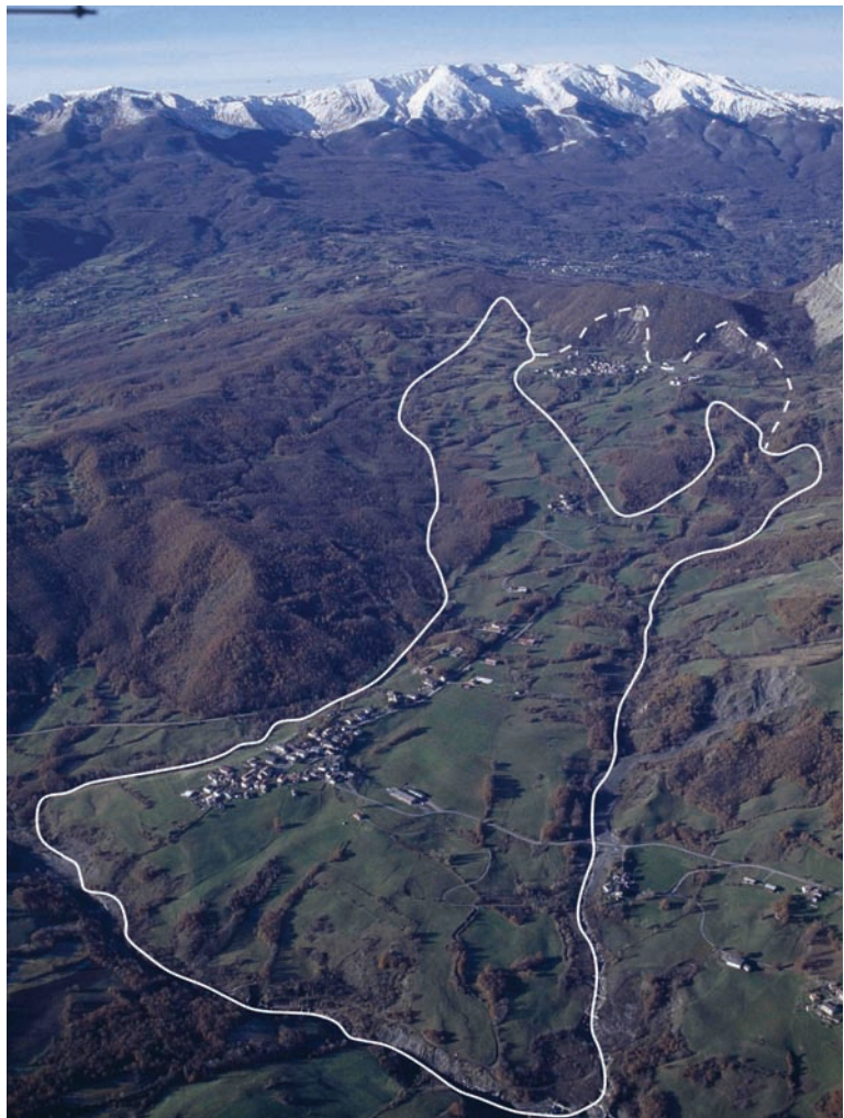
Figure 9. The Morsiano village, lying on a large landslide, symbolises the risk related to ancient landslide bodies. Despite its age (a wood sample found inside it dates back to 13.500 Cal. years B.P) the landslide is still active in several portions, threatening and damaging the village. Reactivations occurred in 1631 (partial), 1651 (total), 1880 and 1959 (partial). Similar situations are quite common in
