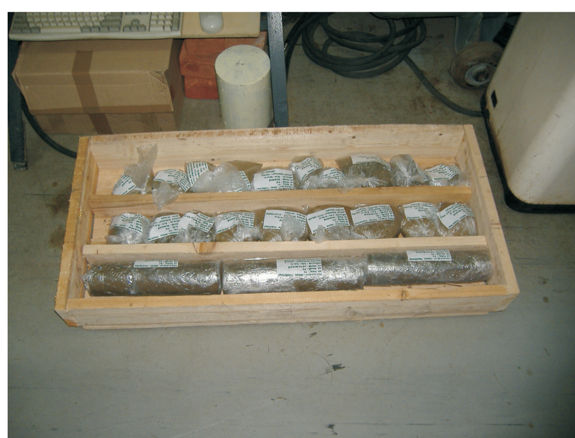
Fig. 2: Recovered drill samples in field box. Directly after the recover from the borehole the samples were wrapped carefully in plastic foil to avoid dehydration and send to the laboratory for Geotechnical testing.
