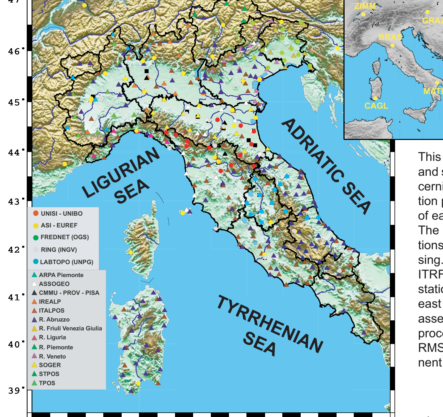
Figure 3. Locations of 289 permanent GPS stations used in this work. Circles and triangles respectively indicate scientific and commercial permanent stations, given in the legend. The inset shows the 6 IGS stations we have used to align the above regional network to the ITRF2005 reference frame.
