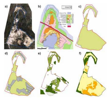
Figure 4: Main intermediate results from geological and environmental studies carried out at the Codaçal ASI: a) aerial view of the Codaçal ASI; b) geological thematic mapping; c) delimitation of the suitable areas for limestone quarrying; d) existing licensed quarries; e) GIS integration of the natural values evaluation process; and f) land use spatial planning proposal for the Codaçal ASI (colours according to Figure 3).
