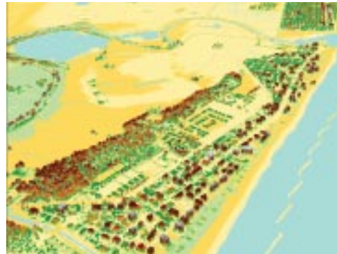
Digital surface model of the mouth of the river Savio, obtained with LIDAR remote sensing.
