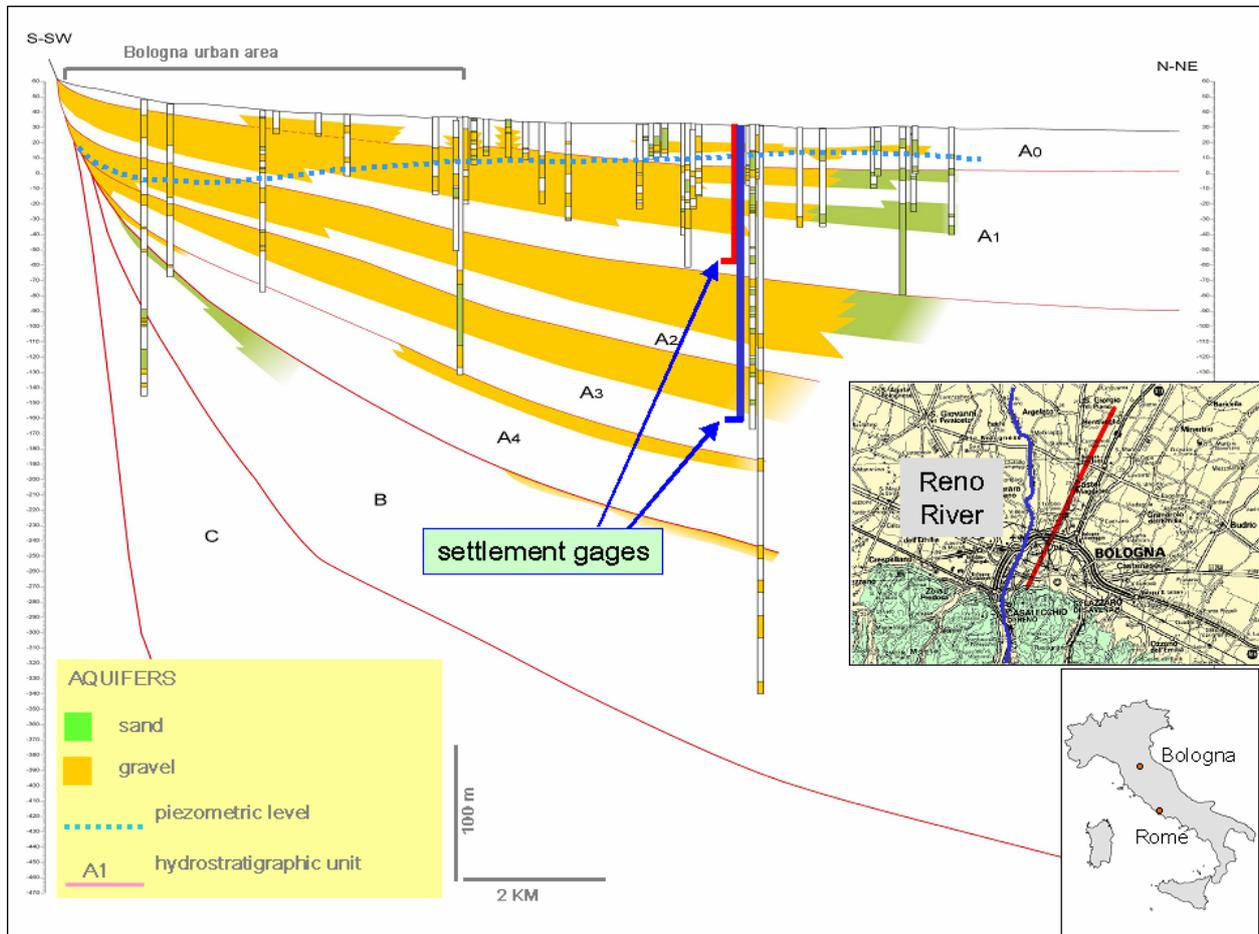
Figure 2 - Geological cross-section (red line in the plain view) describing the subsurface hydrostratigraphic framework and the location of settlement gages for subsidence monitoring. The blue line shows the piezometric level along the section; note the drop due to groundwater pumping in Bologna city
