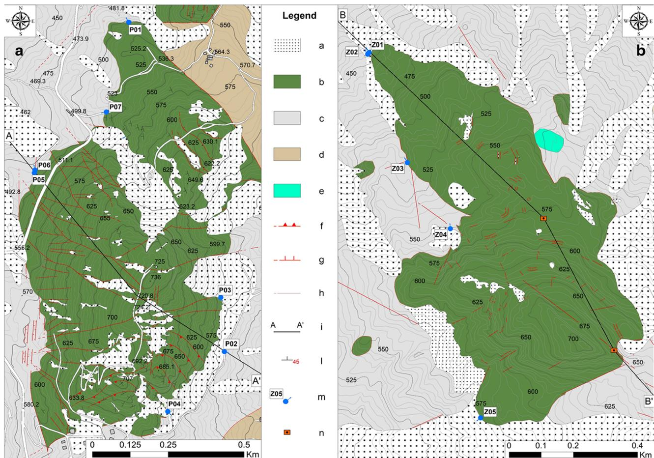
**Fig. 2** Geological sketch maps of **a** Mt. Prinzerza and **b** Mt. Zirone. Legend: a: Quaternary deposits; b: ophiolite hard-rock aquifers; c: poly-genic breccias in clay matrix (aquitard); d: Helminthoid flysch; e:
