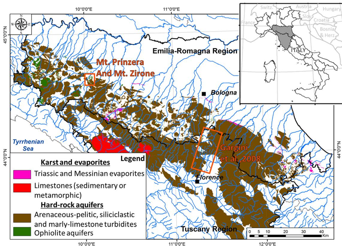
**Fig. 1** Distribution of hard-rock aquifers in the Northern Apennines, Italy. The area of Mt. Prinzera and Mt. Zirone and the area previously investigated by Gargini et al. (2008) are highlighted in orange. Geological
