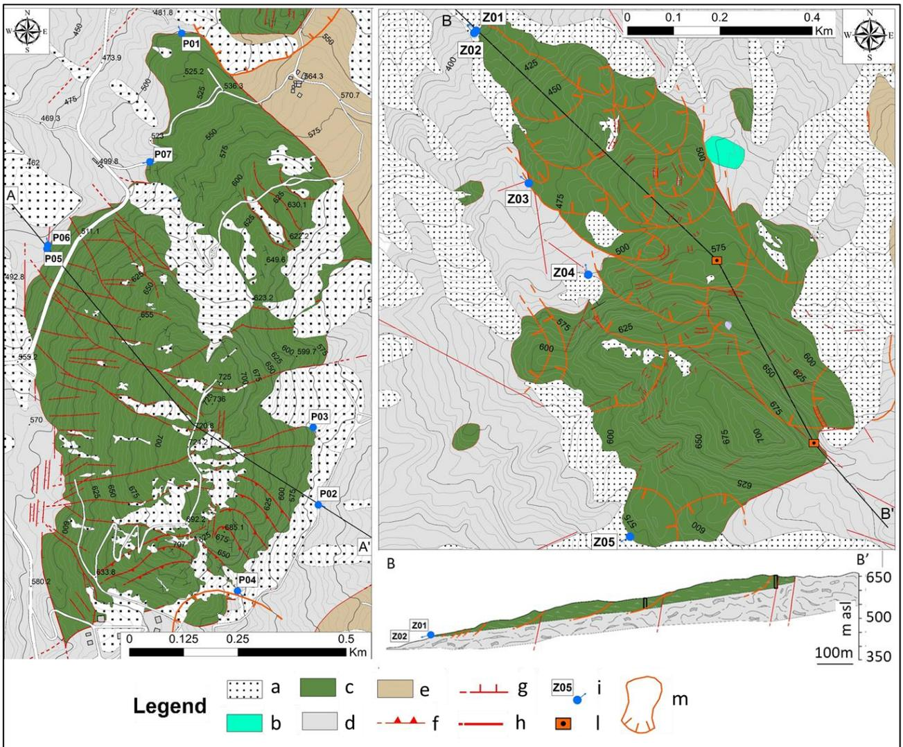
Figure S7 - Geological sketch maps of Mt. Prinzerza (left) and Mt. Zirone (right) a: Quaternary deposits; b: Calpionella limestones; c: ophiolite hard-rock aquifers; d: polygenic breccias in clay matrix (aquitard); e: Helminthoid flysch; f: thrust; g: fault (the teeth indicates the downwards moved side); h: tectonic contact; i: perennial spring; l: borehole; m: rock slope deformation boundary (the teeth indicates the downwards moved side).
