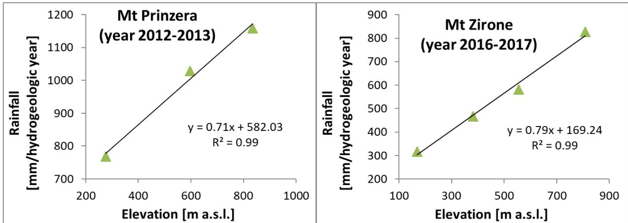
Figure S3 – Linear relationship between the elevation of the meteorological stations and the annual rainfall in the hydrogeologic year of interest.
