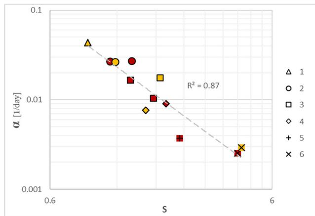
**Fig. 6** Comparison between the coefficient  $\alpha$  of Maillet and the slope  $S$  of the recession plot. The “recession classes” are identified with different symbol shapes. The springs of Mt. Prinzerza and Mt. Zirone are depicted with red and yellow symbols, respectively
