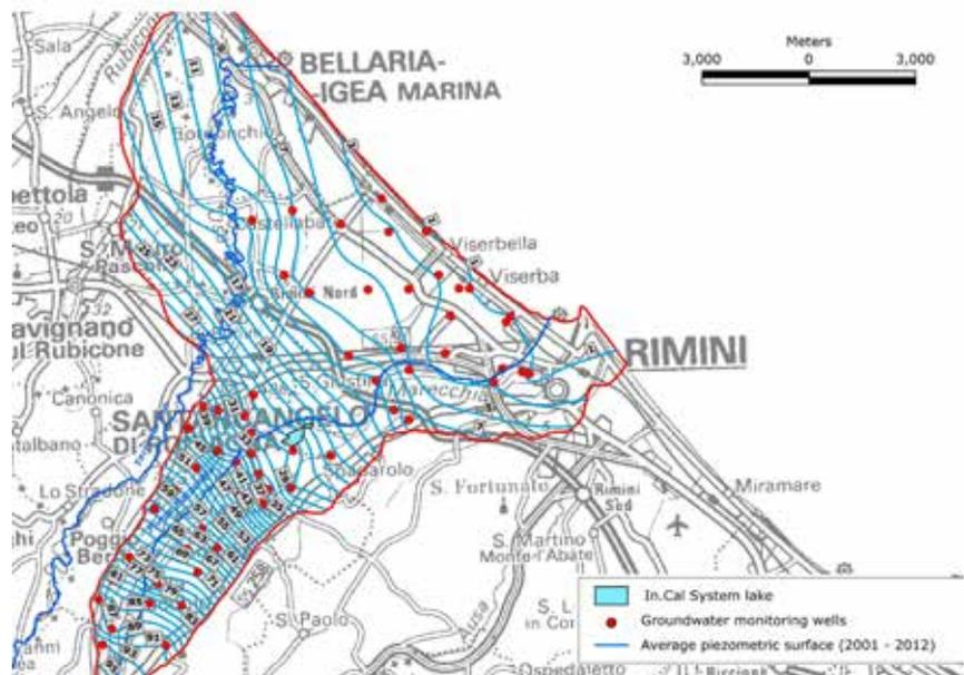
Figure 3: Average piezometric surface of the Marecchia fan (2001-2012).
