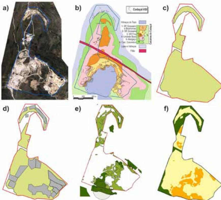
Figure 4: Main intermediate results from geological and environmental studies carried out at the Codaçal ASI: a) aerial view of the Codaçal ASI; b) geological thematic mapping; c) delimitation of the suitable areas for limestone quarrying; d) existing licensed quarries; e) GIS integration of the natural values evaluation process; and f) land use spatial planning proposal for the Codaçal ASI (colours according to Figure 3).
