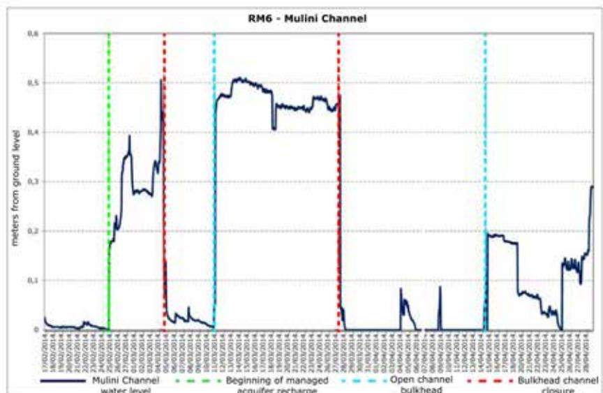
Figure 5: Water level of the channel bringing water to the lake.
