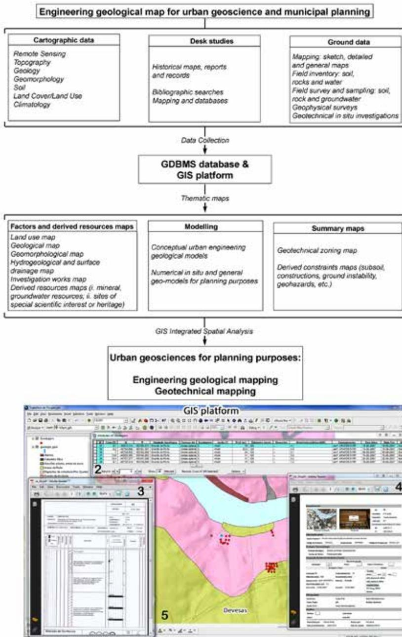
Figure 3: Conceptual flow chart of the engineering geological map for urban geoscience and municipal planning. 1. Application tool to create hyperlinks between features (line, point or polygon) and other files; 2. Database related to ground investigation information; 3. Geotechnical borehole datasheet; 4. Geotechnical inventory datasheet (field and desk data); 5. Detailed investigation works mapping with geological background information.
