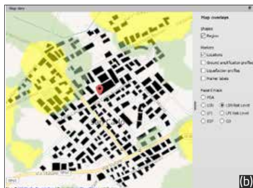
Figure 6: Example of Liquefaction Severity maps in terms of Liquefaction Severity Number (LSN): (a) LSN Risk level quantitative measures; (b) LSN Risk level qualitative classification as defined by Tonkin and Taylor (2013).
