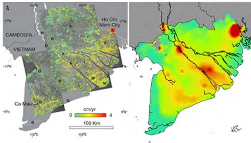
Left: Subsidence rates measured by InSAR for the period 2006-2010 (Erban et. al., 2014). Right: Modelled aquifer-system compaction due to groundwater exploitation (preliminary)
