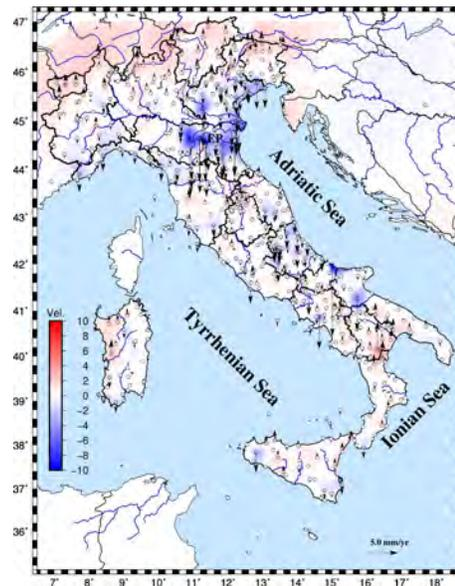
*The present vertical kinematic pattern in the Italian peninsula obtained analyzing the observation acquired from 604 permanent GPS stations. The colours of circles indicate the velocity amplitudes, following the chromatic scale on the map, where the values are in mm/yr. The contour map has been obtained by a geostatistical method over a regular spaced grid (15 Km × 15 Km). EP = Easter Po Plain area.*
