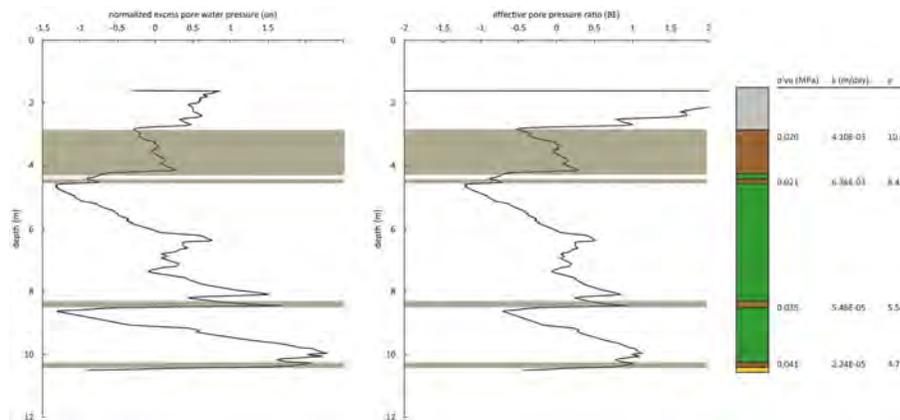
Calculated CPTu values: (left) normalized excess pore water pressure and (center) effective pore pressure ratio, respectively. (right) The corresponding lithological log from the core with effective stress, permeability and void ratio values. Peat is designated with brown shades. When peat is subjected to increasing effective stress, both CPTu values increase, whereas the permeability and void ratio decrease.
