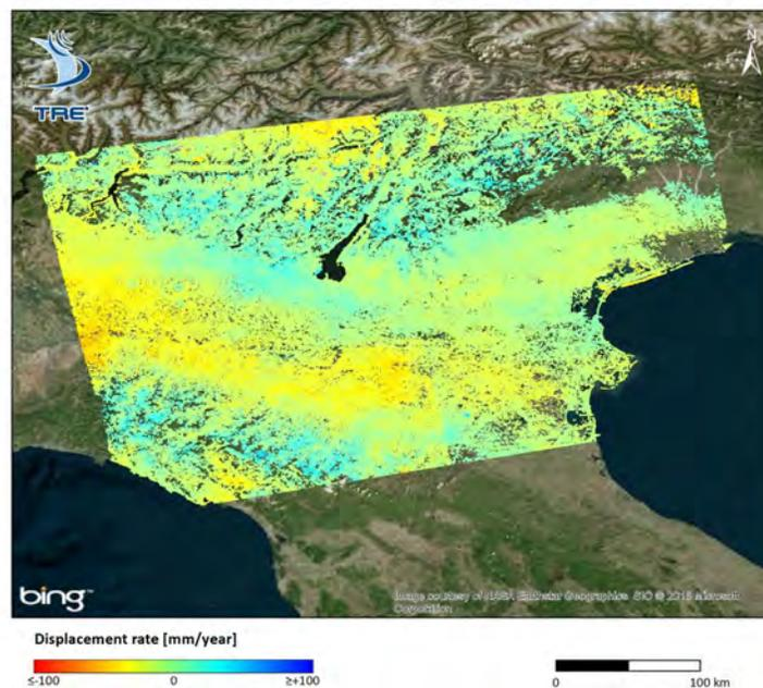
*Example of an Advanced InSAR analysis performed over the North Italy using Sentinel-1 data*
