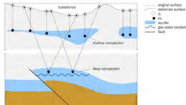
*Schematic view how reservoir compaction influences the surface movement over large areas, and how deep and shallow causes of surface movement interfere at the surface*
