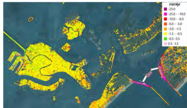
*Average land displacements (2008-2011) of the historical center of Venice and the Lido inlet obtained by PSI on TerraSAR-X images. The MOSE system at Lido inlet consists of two rows of flap gates: 21 gates at the barrier of North Lido (total length 420 m) and 20 gates at the barrier of South Lido (total length 400 m). The barriers are separated by an artificial island.*
