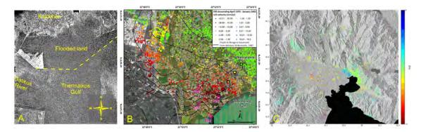
A) Aerial photograph presenting the flooded area after the collapse of the embankment in 1973. B) land subsidence LOS deformation rates from ERS1/2 data (1995-2001), C) PS results from Envisat data (2002-2010) indicating uplift due to ground water recharge
