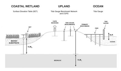
Diagram showing the relationship among vertical land motion recorded by a tide gauge bench mark network on upland (VLMc) and the rod surface elevation table (RSET) method in a wetland (VLMw) [from Cahoon 2015]
