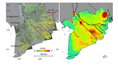
Left: Subsidence rates measured by InSAR for the period 2006-2010 (Erban et. al., 2014). Right: Modelled aquifersystem compaction due to groundwater exploitation (preliminary)
