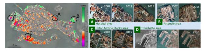
Map of the man-induced displacements experienced in 2013-2015 obtained by removing the C-band (RADARSAT-2) interpolated map from the X-band (COSMO-SkyMed) interpolated solution. The insets show some examples of building restoration
