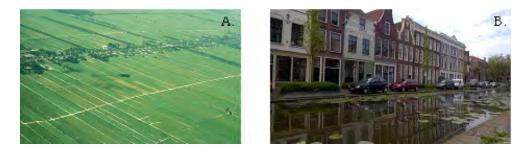
Subsiding peat area in the western part of the Netherlands. A. Rural area (photo: Berendsen). B. Historic city centre of Gouda with water levels that cannot be further lowered without causing oxidation of wooden foundation poles (photo: Erkens)
