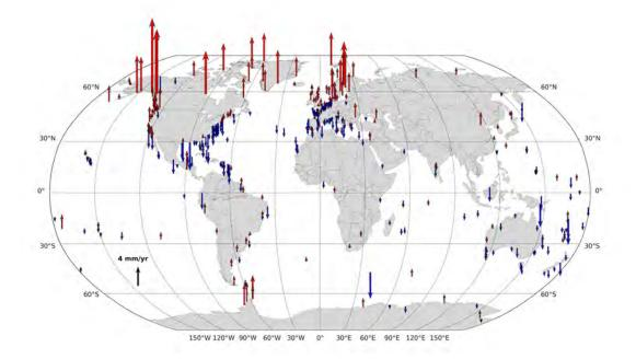
Vertical velocity field from GPS data analysis over 1995.0 to 2014.0 in the ITRF2014
