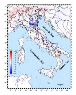
The present vertical kinematic pattern in the Italian peninsula obtained analyzing the observation acquired from 604 permanent GPS stations. The colours of circles indicate the velocity amplitudes, following the chromatic scale on the map, where the values are in mm/yr. The contour map has been obtained by a geostatistical method over a regular spaced grid (15 Km  $\times$  15 Km). EP = Easter Po Plain area.
