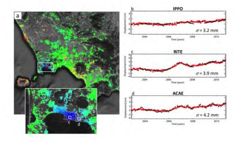
Unsupervised P-SBAS processing chain validation experiments on the Campi Flegrei caldera (Napoli) test site. The three plots show the very good agreement between SBAS-DInSAR (black) and GPS (red) measurements
