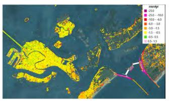
Average land displacements (2008-2011) of the historical center of Venice and the Lido inlet obtained by PSI on TerraSAR-X images. The MOSE system at Lido inlet consists of two rows of flap gates: 21 gates at the barrier of North Lido (total lenght 420 m) and 20 gates at the barrier of South Lido (total lenght 400 m). The barriers are separated by an artificial island.
