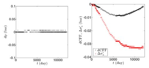
Figure 4.2.11: Change in the pressure and the Coulomb stress (dCFF) at the May 29<sup>th</sup> hypocenter on the Mirandola fault. The pressure change is almost zero because there is no communication between the reservoir and the bottom aquifer. The change in Coulomb stress is very small suggesting no effect of production and injection at the hypocenter in this model.
