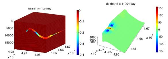
Figure 4.2.8: Changes in pressure in the domain (left) and in the reservoir layers (right) in the case with lateral aquifer support only.
