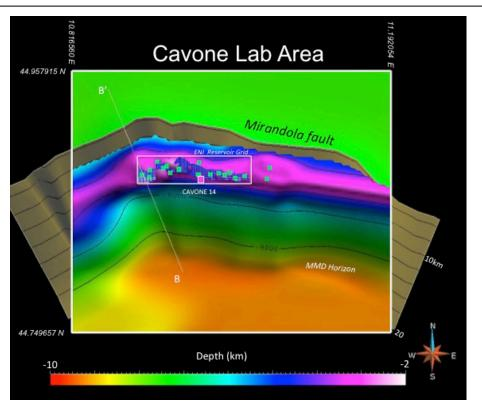
Figure 4.2.1: Map view of the Cavone lab Area, showing depth contours on the top reservoir surface. The small white rectangle shows the extent of the initial reservoir Model, which has been extended to include the Mirandola fault. Section B-B' is shown in Figure 1.2.5.
