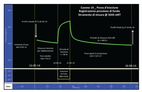
Figure 4.0.3. Detailed record of bottom hole pressure in Cavone 14 during the interference/injection test. Injection was stopped on 15 May, 2014, and kept off except for the 96-hour window from 23 - 27 May, when 600 m3/day was injected.
