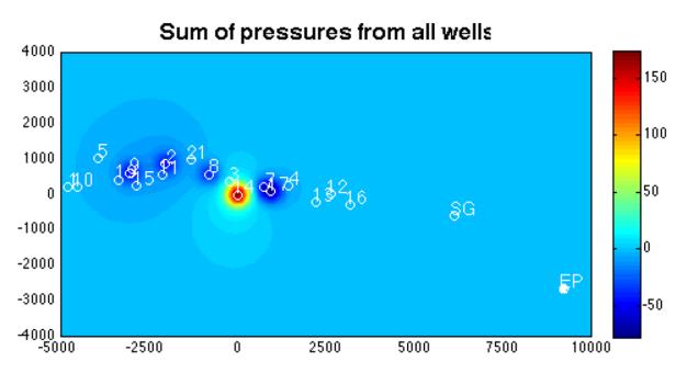
Figure 3.1.3: Calculated pressure field, May 29, 2012, at the top of the Cavone reservoir, assuming a uniform permeability of 0.2 mD. Well locations are given by the white circles, with the epicenter (EP) of the  $M_w$ 5.8 29 May aftershock given by the asterisk. Axes are meters E and N of Cavone 14. Pressure is in bars.
