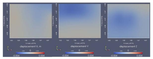
Figure 4.2.17: Displacement field on the ground surface at the end of simulation at t = 11994 day. Pressure depletion in the reservoir leads to subsidence. Left: east-west displacement; Middle: northsouth displacement; Right: vertical displacement. Magnitudes are in meters. Maximum subsidence is less than 3 mm. Notice that subsidence spreads over a larger area of the hanging wall block compared to Figure 4.2.12 because of the pressure drop in the bottom aquifer.
