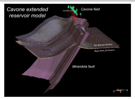
*Figure 4.2.2: Perspective view of the extended Cavone reservoir model, showing the upper and lower reservoir horizons and the Mirandola fault.*
