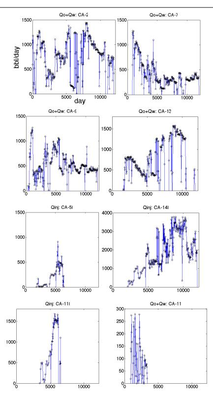
Figure 4.2.7: Liquid flow rates (Qo + Qw) for 5 producers (CA-2, CA-7, CA-9, CA-13, CA-11) and 3 injectors (CA-5I, CA-14I, CA-11I) out of the 19 Cavone wells from the coupled simulation. Wells are able to produce and inject at the historical rates as shown by the good agreement between the dotted curves (historical rates) and the solid curves (simulated rates).
