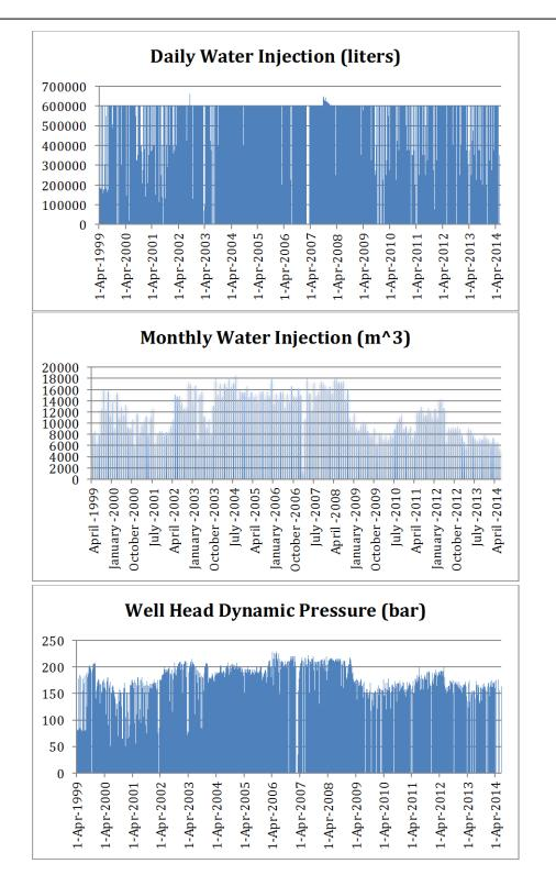
Figure 4.0.5: a) Daily record of the volume of water injected into the Cavone 14 well between April 1, 1999 and June 30, 2014, b) Corresponding monthly record of the volume of water injected into the Cavone 14 well, c) Corresponding daily record of the reinjection pressure at the Cavone 14 well head.
