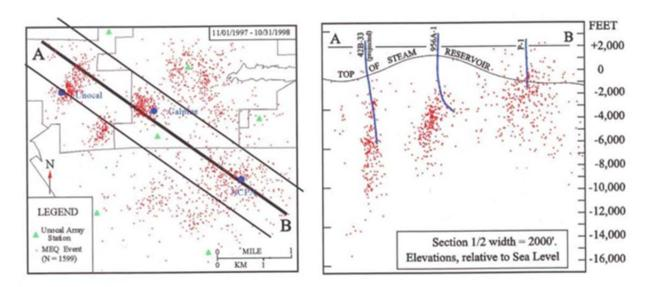
Figure 3.4.1: Seismicity at the Geysers geothermal field, which is located in northern California, USA. Left panel is map of showing location of injection wells (blue) all located earthquakes 1997-1998 (red) and line of cross section. Right panel is cross section showing injection wells and depth locations of earthquakes. Figures from NRC, (2012), source: Beall et al. (1999).
