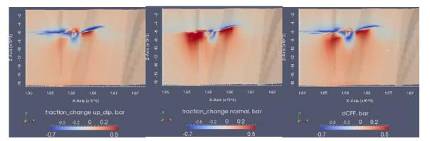
Figure 4.2.15: Changes in the effective tractions and the Coulomb stress (dCFF) on the fault at t = 11994 day for the case with bottom aquifer support. The change in the effective normal traction is positive near producers and negative near injectors because pressure depletion leads to contraction of the reservoir and pressure increase leads to increased compression on the fault. The white cross mark on the dCFF plot denotes the hypocenter location.
