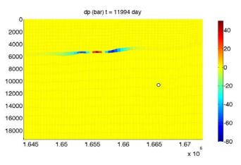
Figure 4.2.9: Change in pressure on the hanging wall side of the fault for the case with lateral aquifer support. The 29 May, 2012 hypocenter location is shown with a white circle. The 20 May, 2012 hypocenter location is on a different fault, for which the pressure changes from reservoir operations is predicted to be zero in this model.
