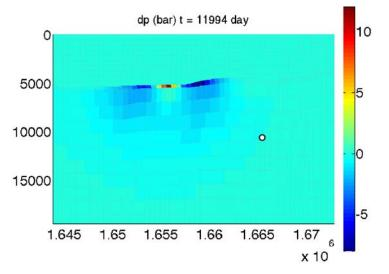
Figure 4.2.14: Changes in pressure (bar) on the hanging wall side of the fault surface. The pressure changes are concentrated in the reservoir layers around the well completions. However, pressure changes diffuse into the aquifer below with time. The 29 May, 2012 hypocenter location is shown with a white circle. The 20 May, 2012 hypocenter location is on a different fault, for which the pressure changes from reservoir operations is predicted to be zero in this model.
