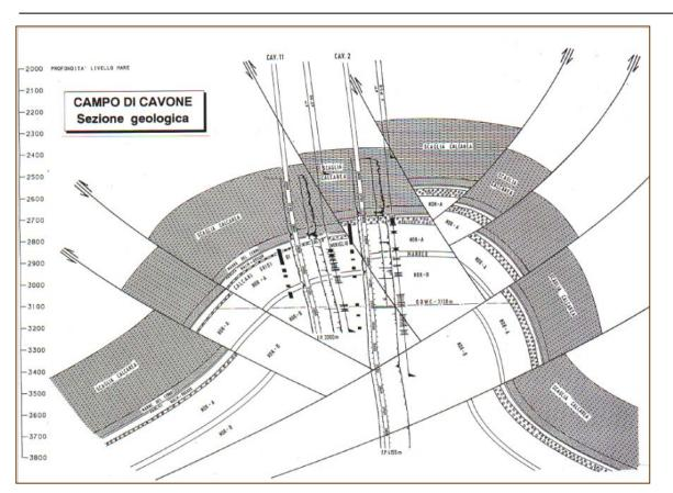
Figure 4.0.2: Cross section through wells Cavone 2 and 11.
