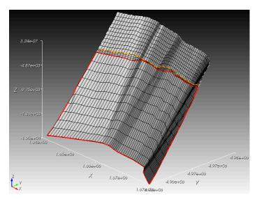
Figure 4.2.4: The Mirandola fault surface in the Cavone geomechanical grid. The reservoir layer, defined by the Breccia top and Nor\_B bottom surfaces, is highlighted.
