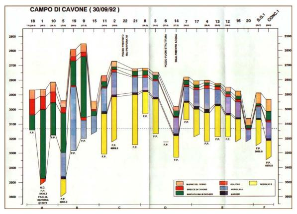
Figure 4.0.1: Stratigraphic columns and correlation for wells in the Cavone field.
