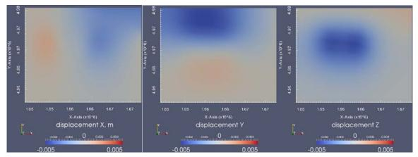
Figure 4.2.12: Displacement field on the ground surface at the end of simulation at t = 11994 day. Pressure depletion in the reservoir leads to formation of a subsidence bowl above the anticline. Left: east-west displacement; Middle: north-south displacement; Right: vertical displacement. Magnitudes are in meters. Maximum subsidence is about 5 mm.
