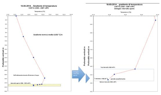
Figure 4.0.4. Profiles of temperature in Cavone 14 as a function of depth below the surface. a) Entire well. b) Zoom in on the region near the bottom of the well.
