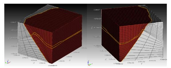
Figure 4.2.3: Cavone geomechanical grid constructed using the three surfaces (Breccia Top, Nor\_B, and Mirandola fault). Red color indicates the hanging wall, and light color the foot wall. The coordinate system is such that the x-axis is easting, the y-axis is northing, and the z-axis is elevation in meters. Left: eastward view, right: westward view of the grid.
