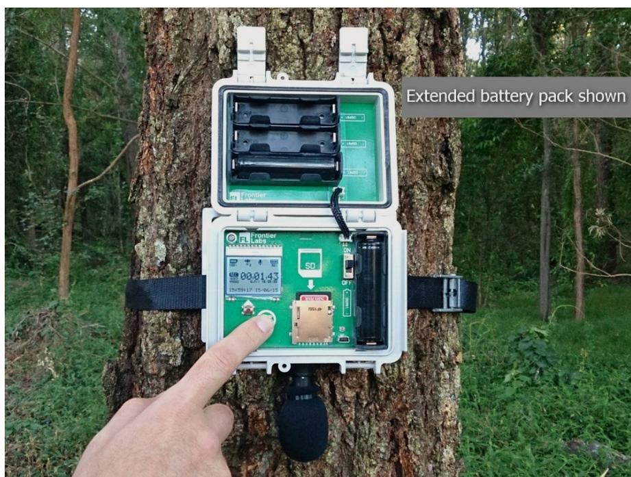
Fig. 44 - Example of installation of bioacoustics recording equipment<sup>90</sup>.
