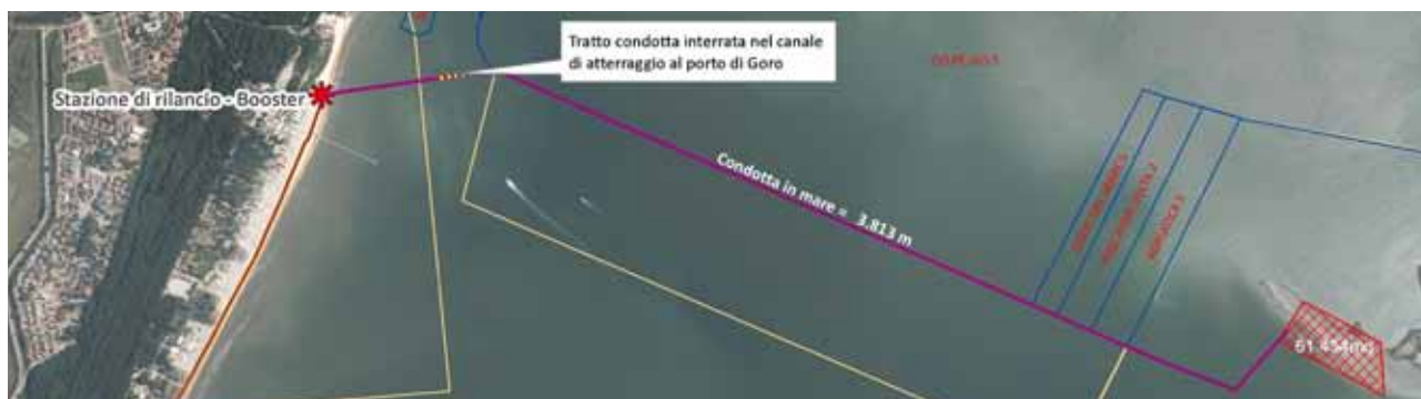
Figure 32 Temporary Sand pipeline of Goro. In red the area of the dredging, the purple line represent the sand pipeline that will be connected to land pipeline (in red).
